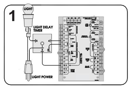
If it is desired that the driveway illuminate when the gate is activated, a light delay timer may be installed. The light delay timer will switch power on to the light for two minutes, then shut power back off. The timer relay is capable of switching up to 10 Amps which will handle most flood or spot lights available. A general hook-up diagram for the light and timer is shown at left.
